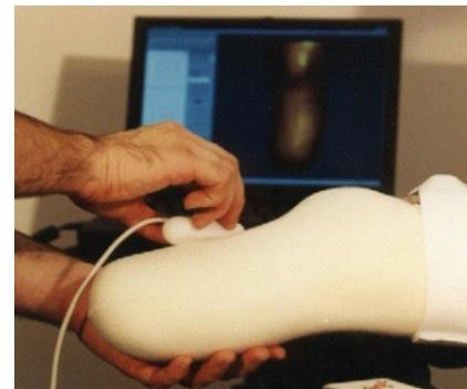
*How it works: A transmitter sends a signal that is picked up by the Tracer Pen and by a sensor that is strapped to the patient's limb. As the clinician moves the pen over the surface of the limb, a control unit determines the location of the Tracer Pen in space and conveys this information to the software.*
