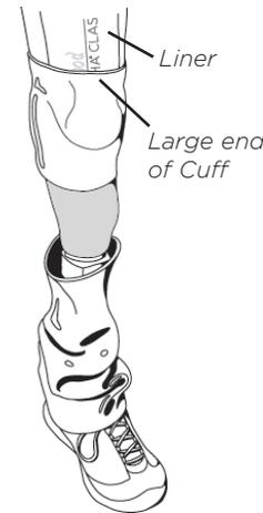
6. Roll the Sleeve up over the Cuff, sealing the Sleeve to the Cuff while also sealing the top of the Sleeve to the liner.
