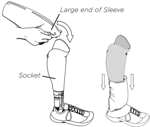
3. Apply the Cuff so that the small end of the Cuff is on the socket, and the large end of the Cuff extends approximately 3 to 5 cm above the highest edge of the socket.
