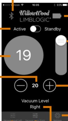
If two pumps are paired with the app, tap the left or right indicator to select which pump to control.
